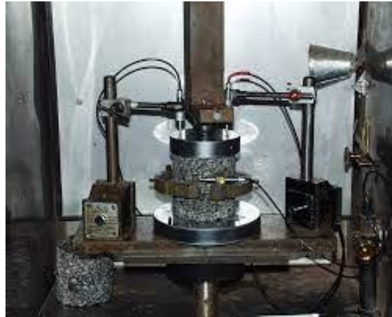
Figure 4.24: Principle of Uniaxial Cyclic Compression Test Under Confinement
