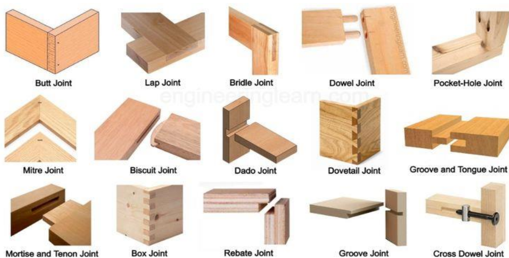
Figure I.11: Joints used in solid wood
