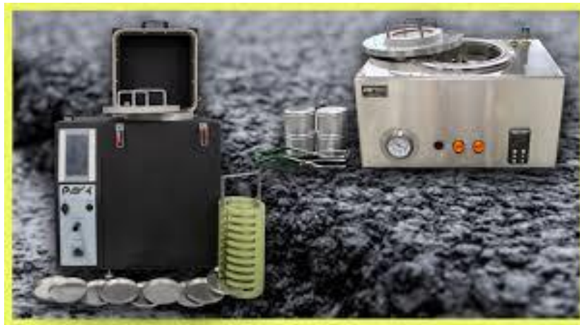
Figure 4.14: The Pressure Aging Vessel test
