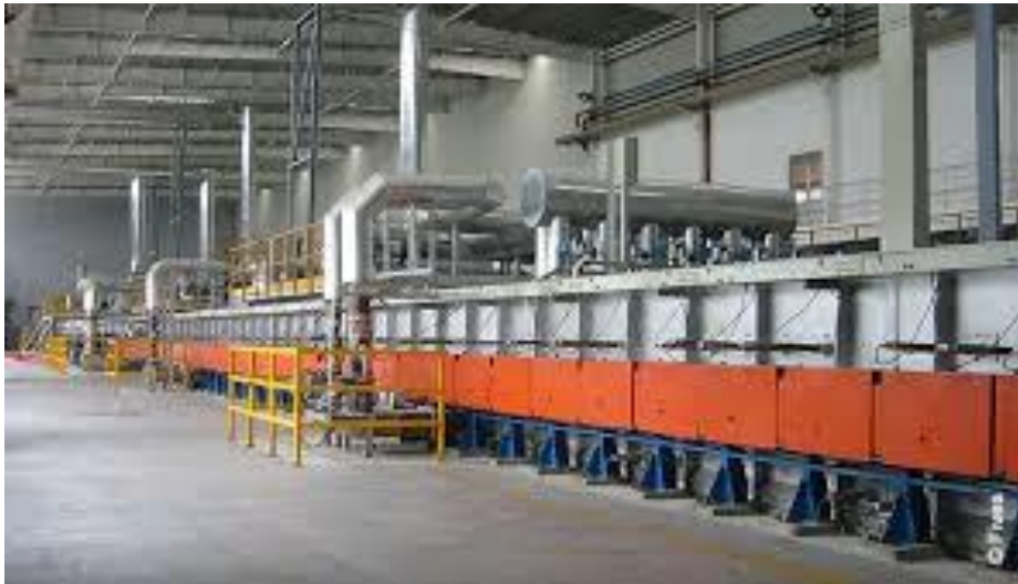
Figure 2.11: Annealing and Controlled Cooling
