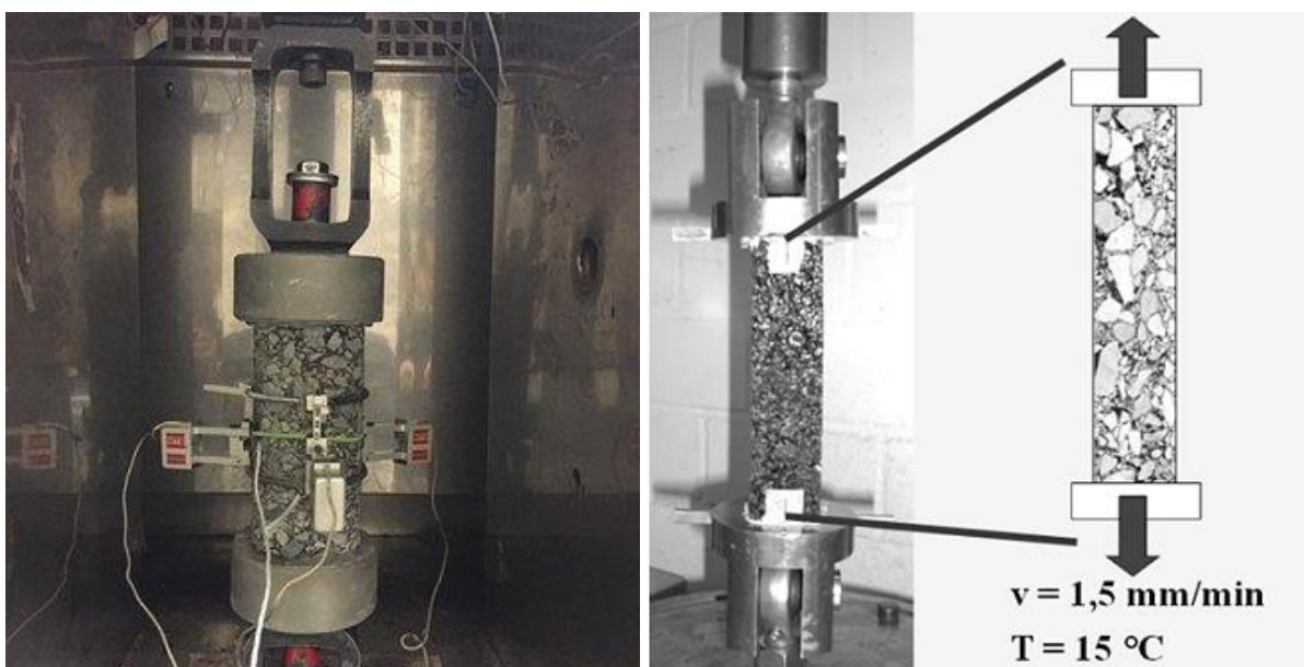
Figure 4.23: Principle of the Direct Tensile Test
