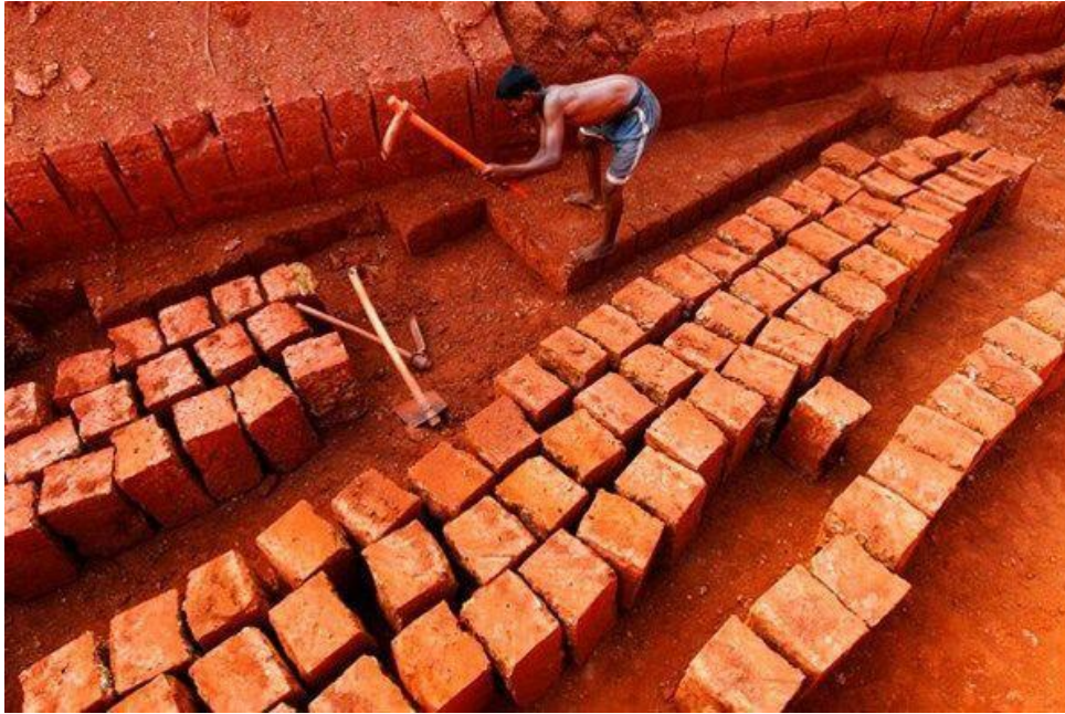
Figure 6.16: Cut blocks extraction
