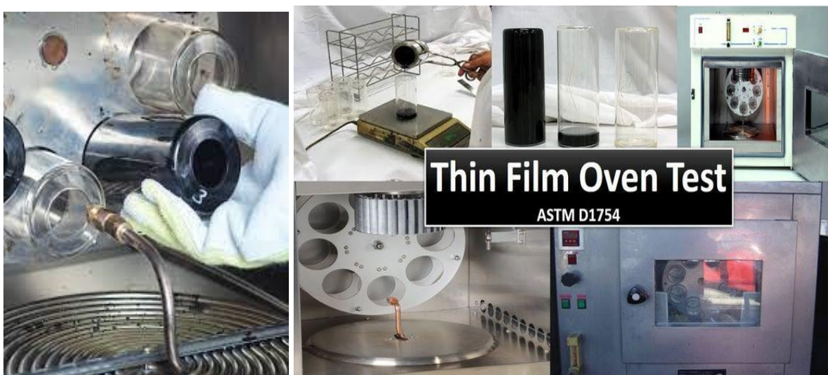
Figure 4.13: The RTFOT test
