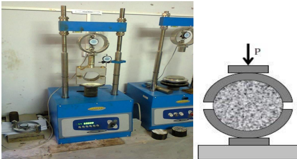
Figure 4.19: Principle of the Marshall Test
